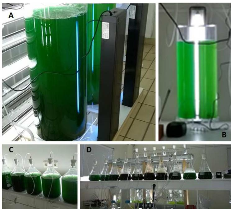
**Figure 4.** Overview of upscale cultivation, comprising different volumes of 2 L and 5 L flasks and 5 L bubble columns (B, C, D) as well as experiments in the two 100 L PBRs (A).
